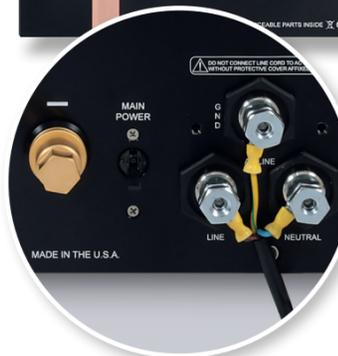
**ABOVE:** Custom loudspeaker terminals are supplied with a special tool to crank them tight against spade or bare wire terminations [the same tool is used to bolt-down the AC mains cable – see left]. A single balanced XLR input is fitted
